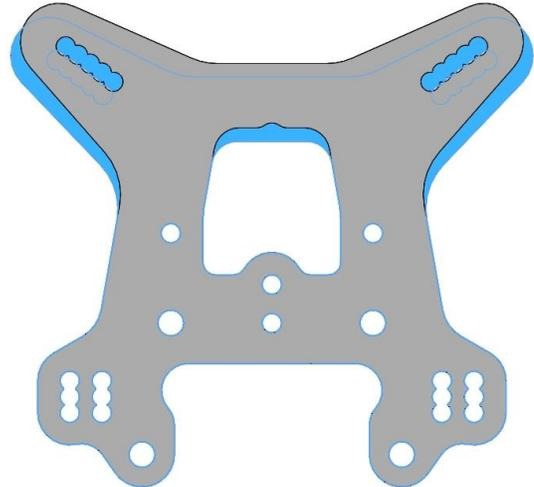
*Difference between new #91422 tower (gray) and standard tower (blue). Shock tower holes are higher.*
